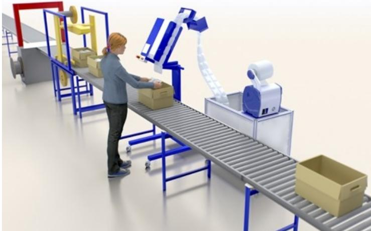
Multiple MINI PAK'R's at one single point offer different air cushions types to accommodate any kind of packing application, and our PRO PAK'R with Speedfeeder rapidly produces the
